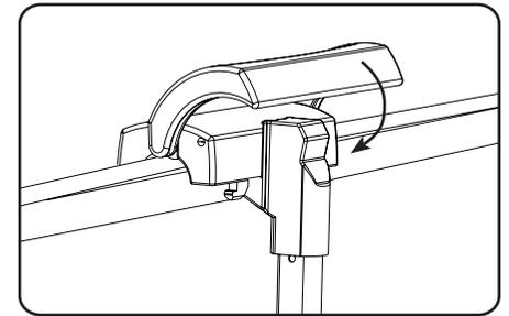
6. Extend the Support Rod to the desired viewing position and lock into place. The screen can be levelled using the adjustable feet.
