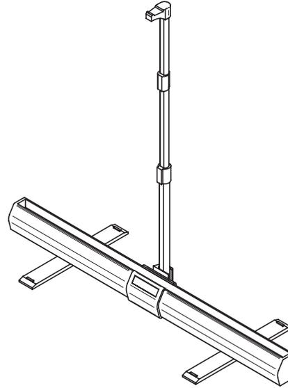
4. Pull the screen up and hook into the top of the support rod.
