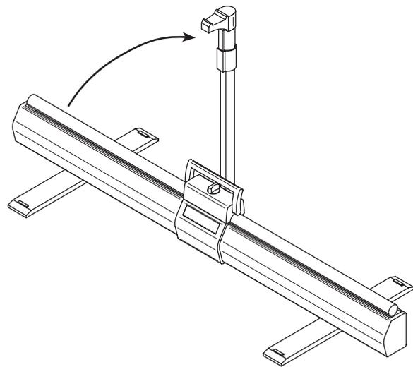
3. Extend the support rod to the desired height and lock into place.
